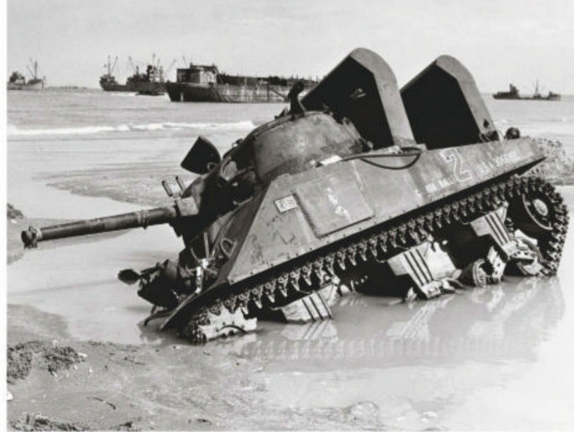
A stranded Sherman nicknamed "Cannon Ball" on Utah Beach. Note the special air intakes for semi-submerged landing
